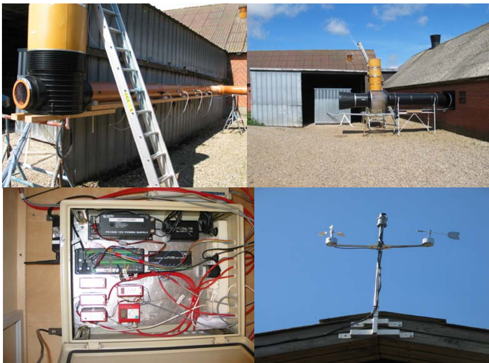
Top left – the research model. Top right – the industry model. Bottom left – the data logging unit. Bottom right - the weather station with wireless communication facilities.
