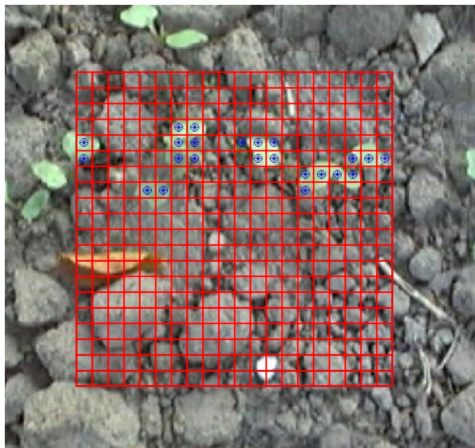
Figure 1. The computer vision system takes pictures from the field surface. In each picture the area of interest is divided into square cells (□) of e.g. 0.25 by 0.25 cm each. Cells containing at least 50% weed leaves are marked for spraying (⊗).
