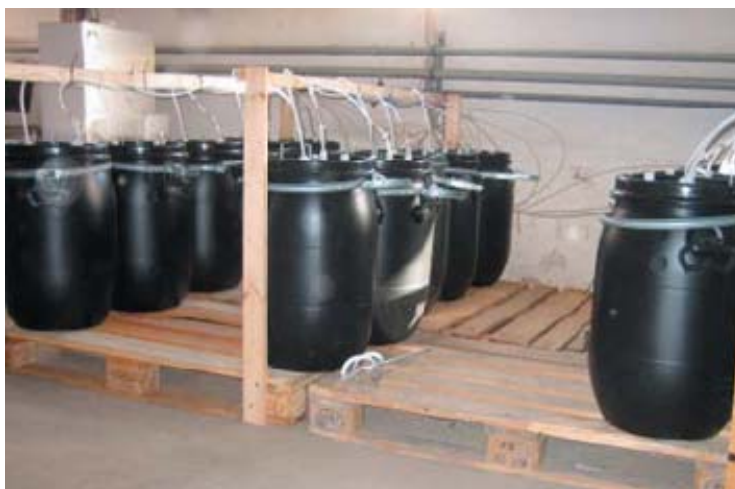
Experimental set-up with dynamic emission chambers including air supply to and exhaust from head space above the slurry.
